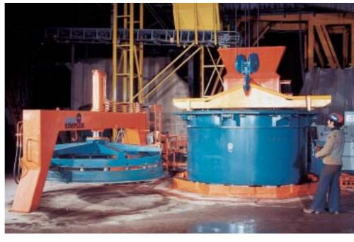
The VIHY Modul Simplex is manually operated, but with electrically or hydraulically powered operations. Reinforced and non-reinforced pipes, circular or non-circular pipes with or without socket, with or without prebed, manholes, tapers, jacking pipes, box culverts, as well as PE-lined and PVClined pipes can be manufactured with this machine. The dimension range goes up to ø3600 mm depending on the machine design chosen.
